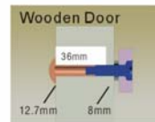
Wooden Door Drill a hole Inside: Diameter is 8mm Outside: Diameter is 12.7mm
