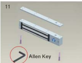
11 Use Allen Key to screw the lock body on the mounting plate.
