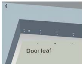
4 Drill holes on the marked positions
